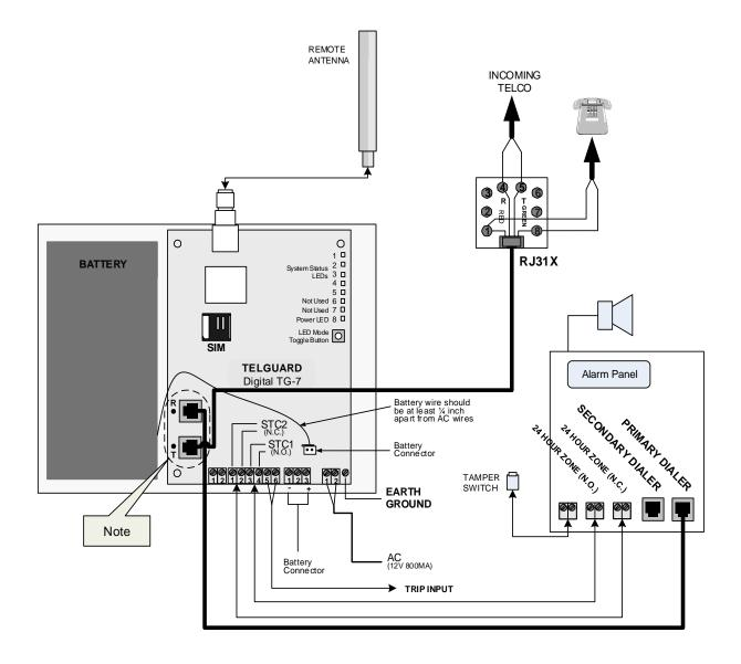
Note: When using this scenario, the programming of the TG-7 is what determines whether the TG-7 is meant to work as a back-up or primary communicator.
